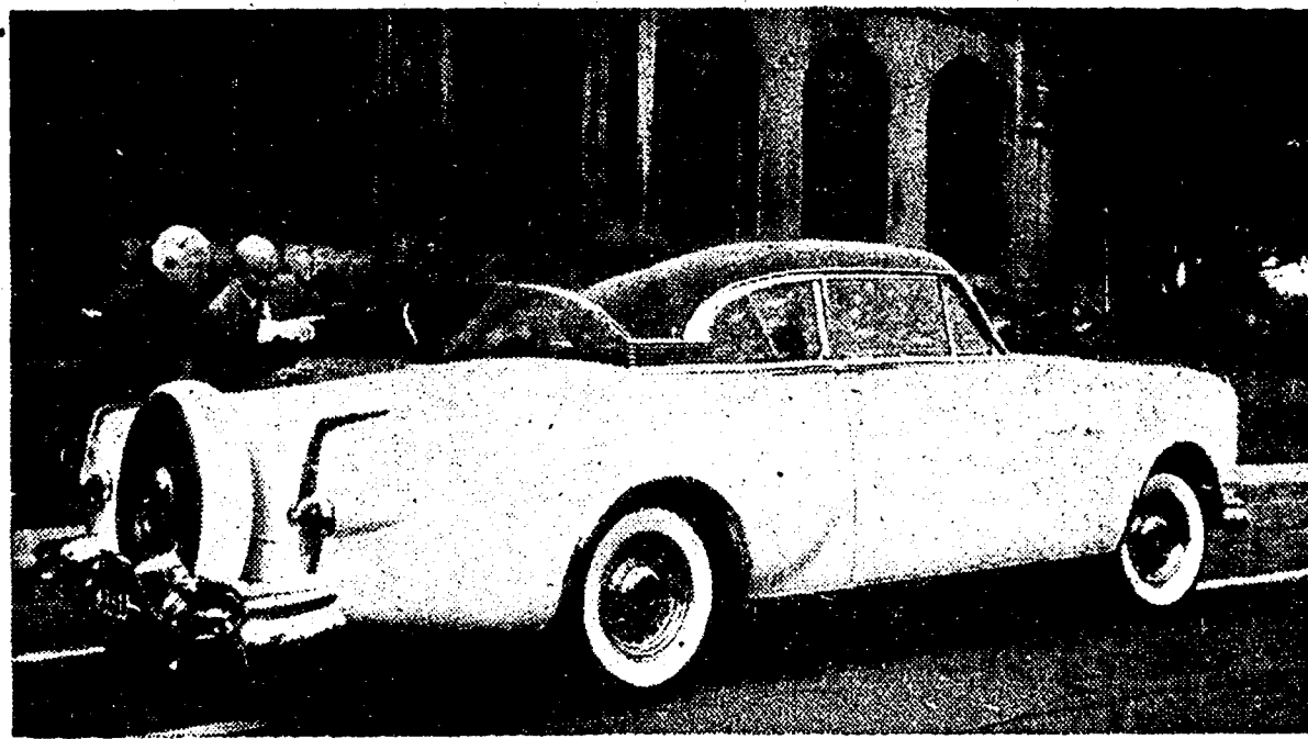
This is the "Balboa," a new experimental sedan with sharply different design aimed at passenger comfort which has been developed at Packard Motor Car Co. A completely new feature of the car is the styling of the rear window which has a reverse slope and is covered by a canopy.
