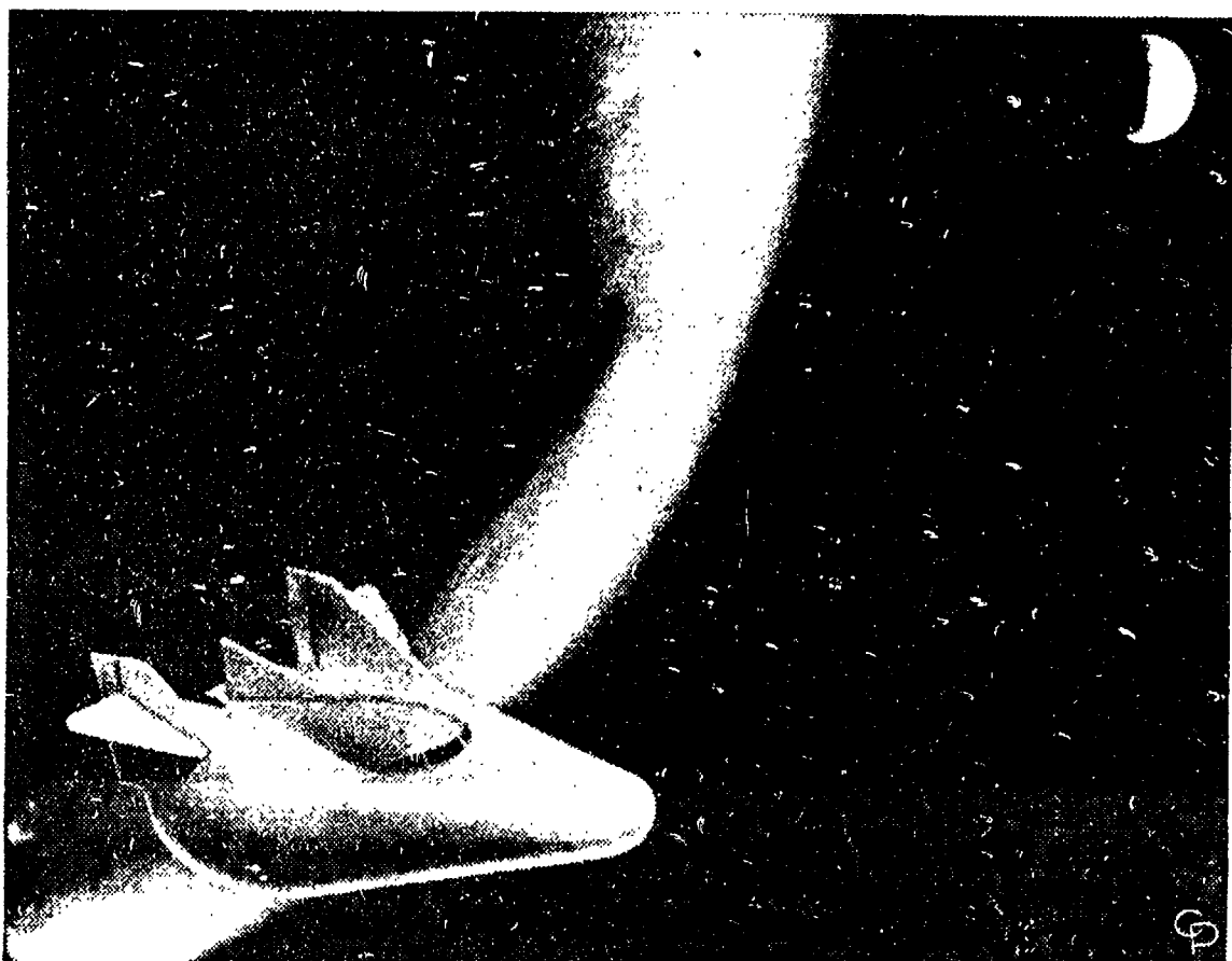
'LIFTING BODY,' IT'S CALLED—From Moffett Field, Calif., comes this sketch of the manned, wingless space vehicle M-2 "lifting body," depicted in a probable mission as it leaves the vicinity of the Earth to rendezvous with a space station. It was conceived and proved feasible by scientists at NASA's Ames Research Center. The "lifting body" is intended to attain aerodynamic stability and lift from a body alone, eliminating need for wings, and can be landed like a conventional airplane.
