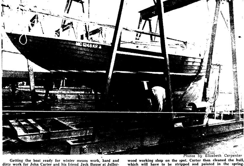
son Beach Marina. After pulling into a dock the mast was cradled or removed, and the boat was hoisted out of the water where a custom-built wooden cradle was put together in the
