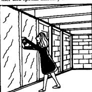
FIGURE 3 Homeowner presse CertainTeed's fiber glass studs with the kraft facing towards the air conditioned area of the home and staples to the
