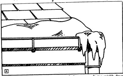
ICE DAMS, OR ICE BUILD-UPS, are caused when snow melts too quickly down your roof and freezes at the cornice. They can be prevented via adequate insulation and ventilation.
