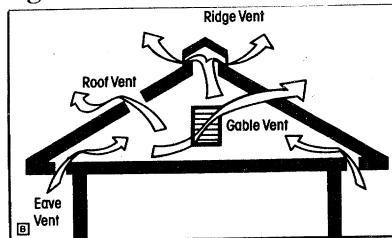
PHOTO ILLUSTRATES the four most common types of ventilation.
