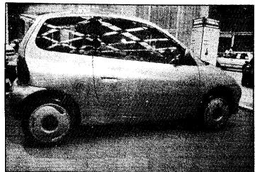
B. Volkswagen brought its wee Chico 2 plus 2 hybrid-powered concept car to Detroit. It features a fully-automatic switchover (at 37 mph) between gasoline power and electric
