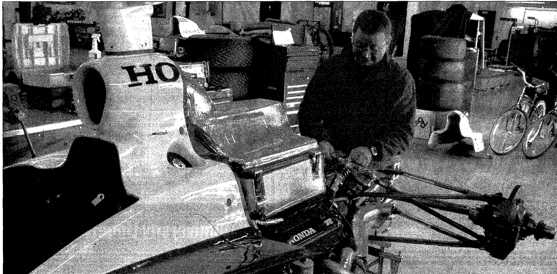
Robbie Buhl, left, monitors practice last year at the Indianapolis Motor Speedway. At Dreyer & Reinbold Racing headquarters, above, mechanic Nick Allen covers a brake line with an aerodynamically shaped strip of carbon fiber. Engineer John Dick, below, tends rear suspensions components.
