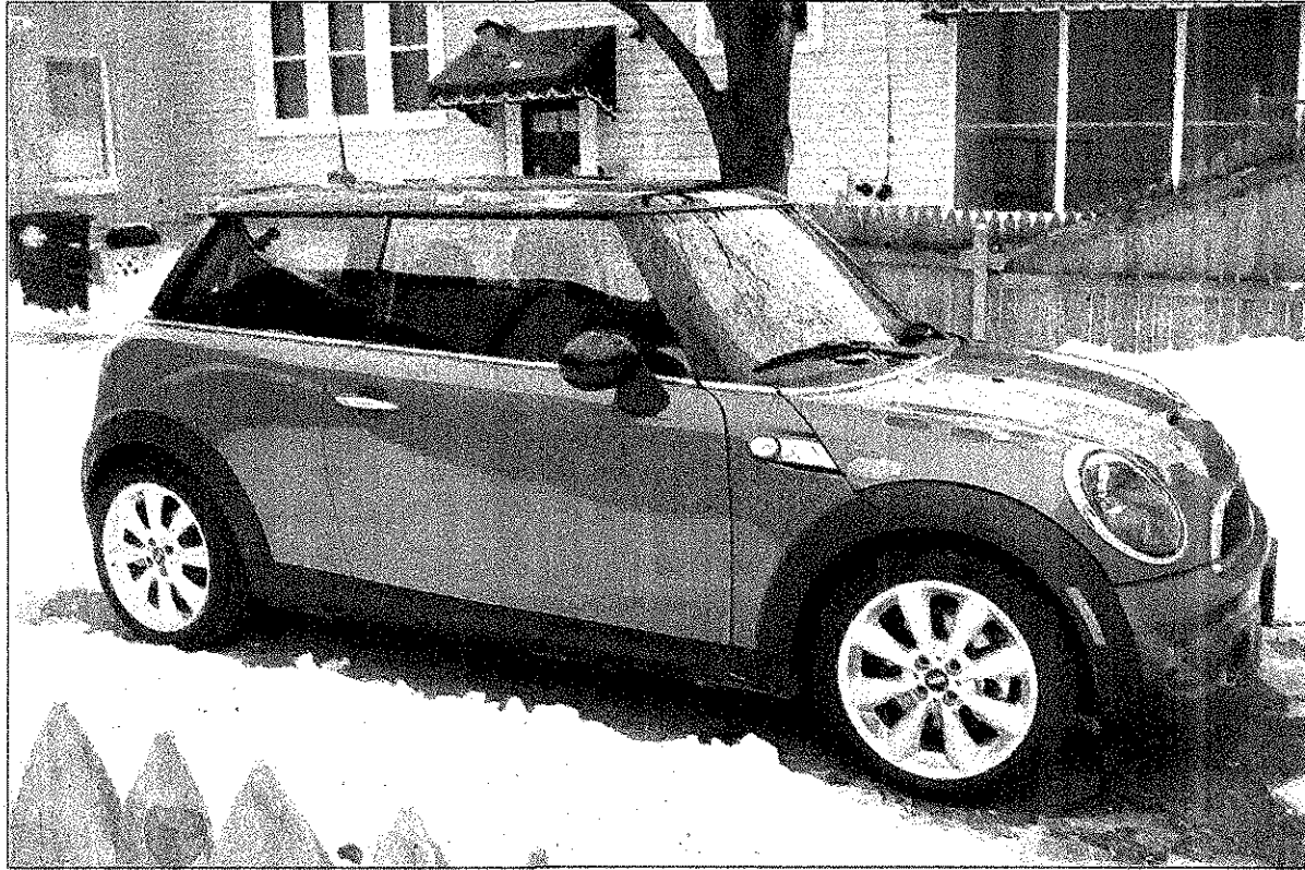
The 2011 Mini Cooper and Cooper S share a 1.6-liter four, but the S model includes turbocharging that spikes horsepower from 121 to 181. An enormous speedometer reminds the Mini driver of a heavy foot; it also encircles an information screen.
