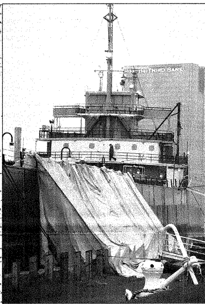
Bare metal on the first of many hull sections to be stripped and repainted.
