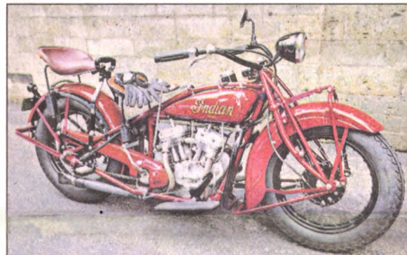
A 1928 Indian 101 Scout motorcycle was built with a longer wheelbase and lower seat height, noted for its handling and used by racers and in stunt exhibitions.
