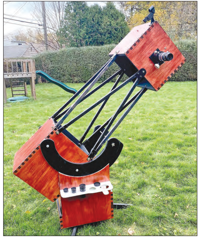
The telescope is made to be collapsible, allowing it to be transported easily for future trips to dark sky parks.
