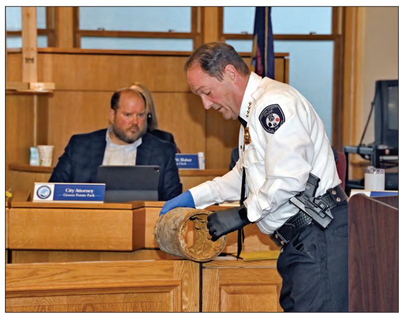
Grosse Pointe Park Director of Public Safety Bryan Jarrell shares with city council an example of old cast-iron pipe occluded with tuberculation.
