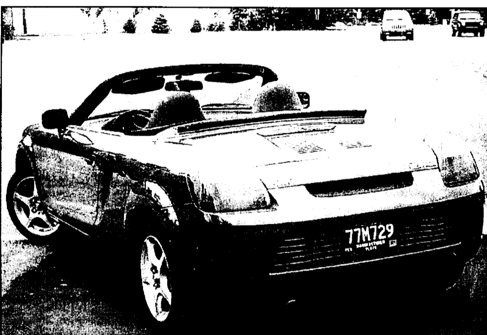
From the rear, the Toyota MR2 Spyder retains its exotic look. The engine is behind the seats, ahead of the rear axle, which is good for balance, bad for cargo space.
