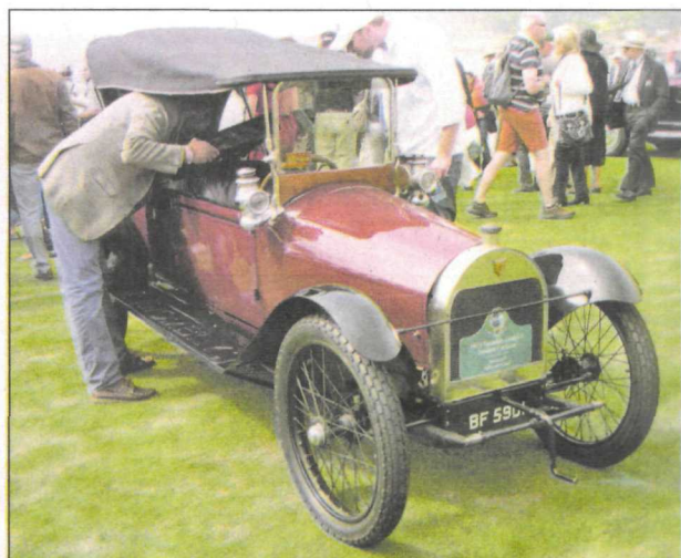
Built in Pennsylvania, this 1913 Twombly Model A chain-driven Tandem with friction drive was shown by owner Peter Russell of Pulborough, England.
