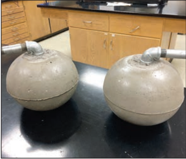
Students created their own curling stones out of salad bowls, concrete and a galvanized plumbing pipe.
