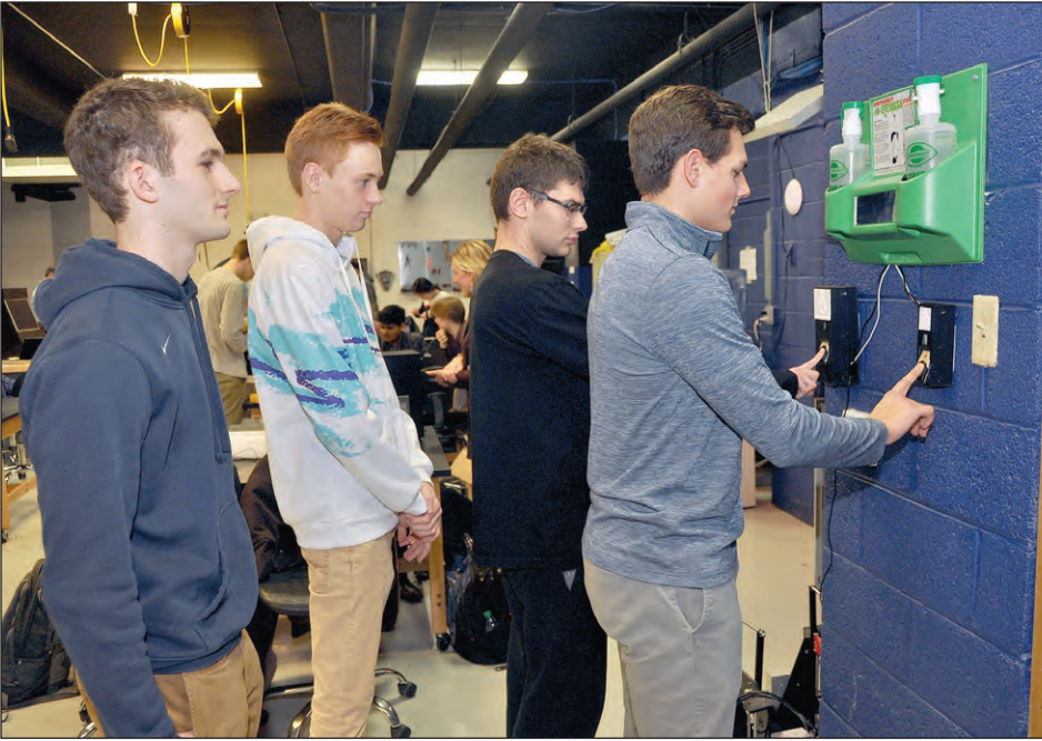
From left, Alex Bower, Austin Wright, John McInchak and Wyatt Dennis designed a biometric attendance scanner for teachers to track attendance. To accommodate multiple users arriving to class at once, the team built a second, smaller version of the scanner connecting to the larger one, which contains the Raspberry Pi, a low-cost, credit card-sized computer. The total cost for both is approximately $150. An industrial version would run more than $400.
