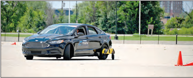
Teens learned to turn into a skid; the wheel brace on the back of this car helps stabilize the vehicle when skidding on icy or wet pavement. This teaches students how to control the vehicle in case of a skid.
