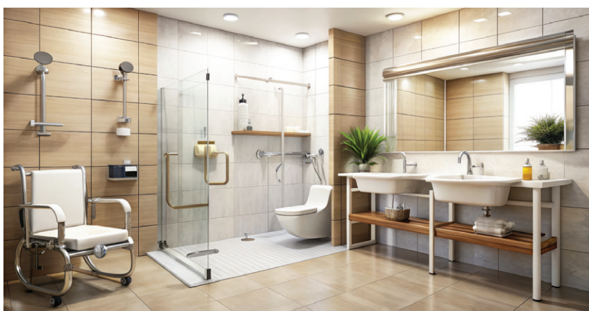
A zero-step walk-in shower, above, provides easy access for seniors who have difficulty with knees or hips. The flat entry and seating accommodate mobility issues.
